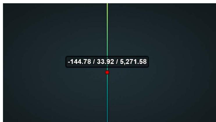
Figure 3-8: Point cloud is pressed together due to an insufficient decimal precision.
