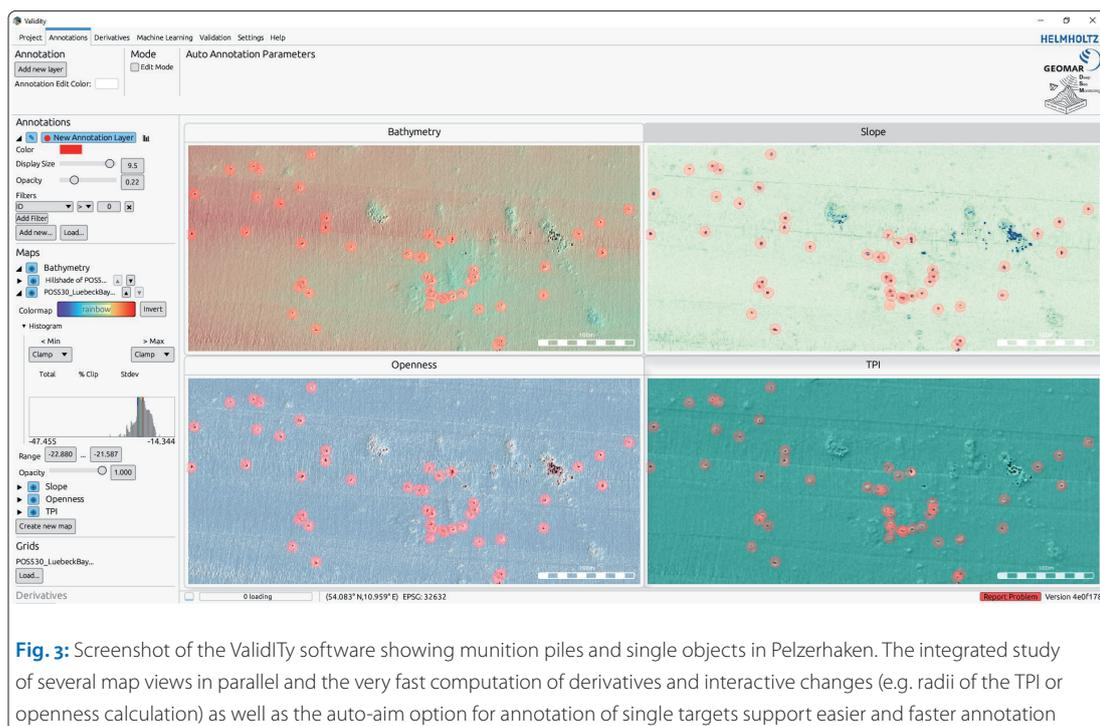
**Fig. 3:** Screenshot of the ValidTy software showing munition piles and single objects in Pelzerhaken. The integrated study of several map views in parallel and the very fast computation of derivatives and interactive changes (e.g. radii of the TPI or openness calculation) as well as the auto-aim option for annotation of single targets support easier and faster annotation
