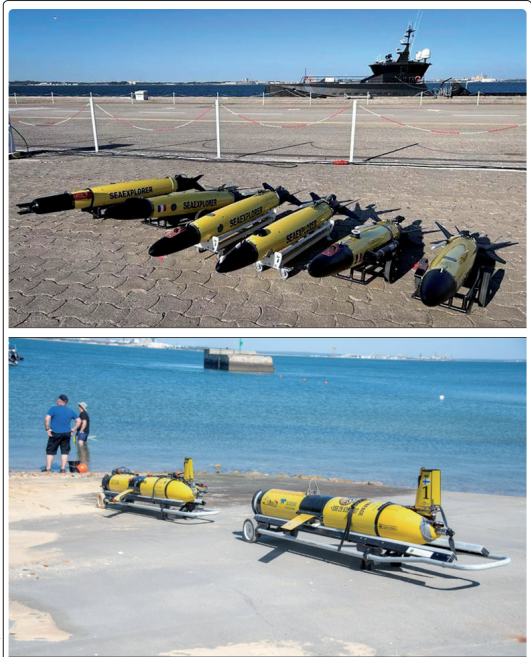
Fig. 6: Examples of gliders deployed during REPMUS24. Top: Alseamar SeaExplorer. Bottom: Teledyne Slocum
