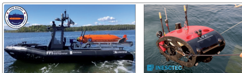
Fig. 9: Assets employed in REPMUS24 CUI scenarios: KD HUGIN 3000 (left) and INESC TEC EVA (right)
