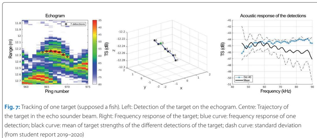
Fig. 7: Tracking of one target (supposed a fish). Left: Detection of the target on the echogram. Centre: Trajectory of the target in the echo sounder beam. Right: Frequency response of the target; blue curve: frequency response of one detection; black curve: mean of target strengths of the different detections of the target; dash curve: standard deviation (from student report 2019–2020)
