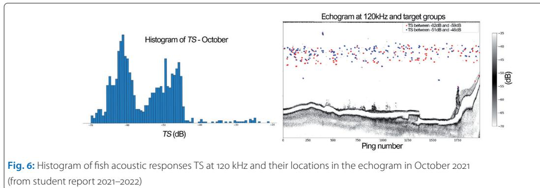
Fig. 6: Histogram of fish acoustic responses TS at 120 kHz and their locations in the echogram in October 2021 (from student report 2021–2022)
