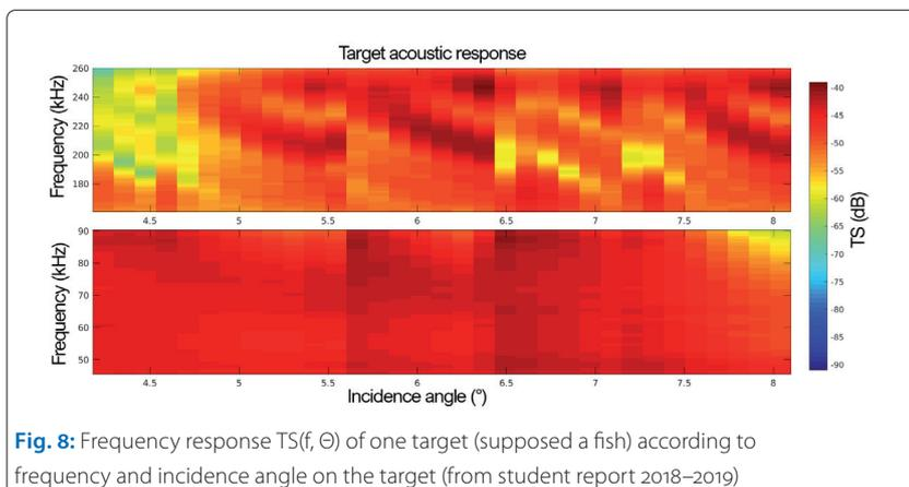
**Fig. 8:** Frequency response  $TS(f, \theta)$  of one target (supposed a fish) according to frequency and incidence angle on the target (from student report 2018–2019)
