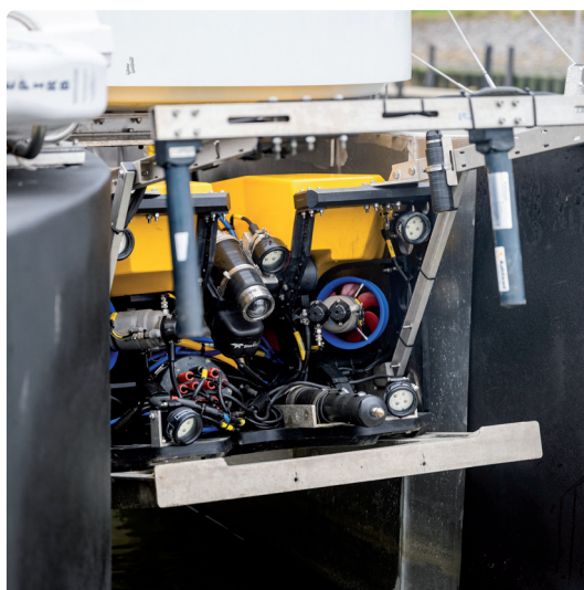
Fig. 2: The eROV which is docked on the USV and controlled through the remote operations centre can be automatically deployed and retrieved from the water
