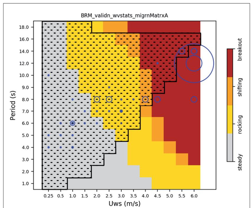
**Fig. 5:** (Colour grid) Matrix of simulation results by wave bottom orbital velocities and periods. It shows the largest motions possible for BRM objects under the varying conditions: larger object displacements from the yellow to red zones. (Stipple) Superimposed wave climate of the German Bight – same as Fig. 2. (Blue points) The validation data, with the symbol size representing actual displacements observed for BRMs and similar objects, in various worldwide studies
