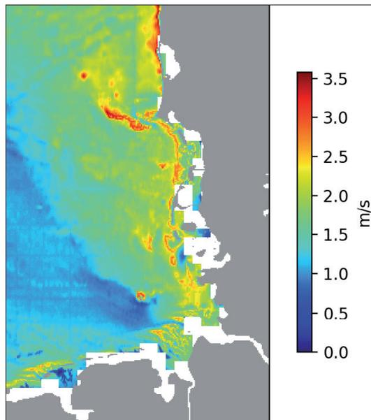
**Fig. 3:** Near-bottom wave-induced flow velocity amplitudes (m/s) during a severe event in 2018, calculated from Wavewatch III data. The high values (red) tend to coincide with shallow-water areas. (Blank areas are not covered by the wave statistics.) During the event sea-surface significant wave heights ( $H_s$ ) attained 6 to 9 m over much of the area
