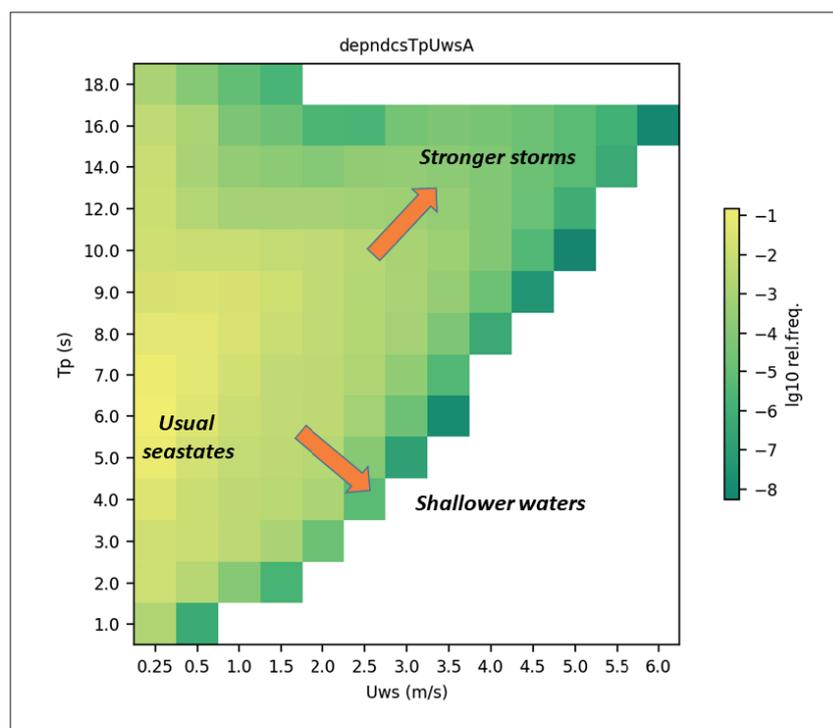
**Fig. 2:** The total population of wave-induced bottom-velocity amplitudes ( $U_{ws}$ ) and periods ( $T_p$ ) in the German North Sea, based on 20 months of Wavewatch III data. The population is over all spatial pixels \* time slices. Yellow areas are »usual« conditions and the arrows show important trends in the data. Note the prevalence of events with storm severity, approximately  $U_{ws} > 2.5$  m/s
