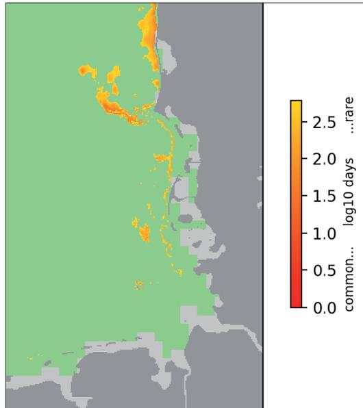
**Fig. 6:** Migration potential in terms of return times on significant movements for a BRM-type object, computed with 20 months of wave data. Movement is forecast in the orange areas for return times of months to years. (Pale green – no indications of movement. Grey marine areas – no wave data available)
