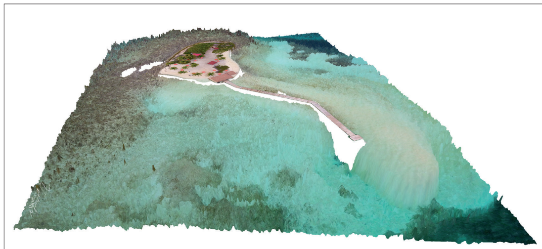
Fig. 3: Combining drone- and satellite-analysis for mapping shallow water environments. The example shows an area of approximately 250 × 250 m in Belize and represents depth at 9 cm spatial resolution overlaid with a real-colour image which shows the different seafloor types from bright sand to coral and hardbottom areas (top left) to sparse to dense seagrass areas (lower right and centre)
