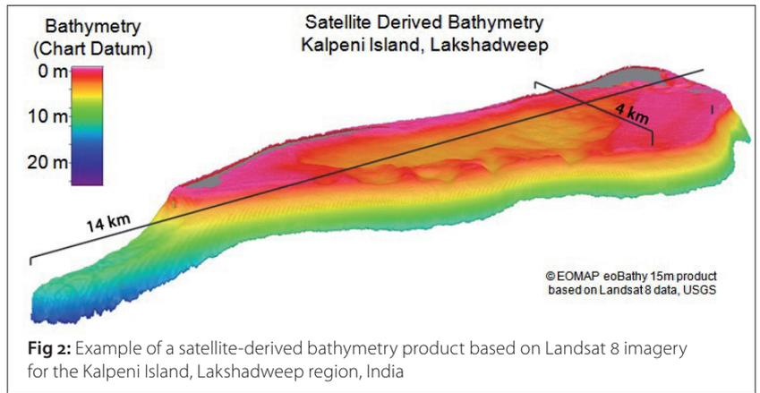
**Fig 2:** Example of a satellite-derived bathymetry product based on Landsat 8 imagery for the Kalpeni Island, Lakshadweep region, India
