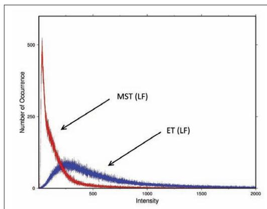
sonars. The curves have similar shapes, in general, but it can be noticed that a kind of scaling factor is present. The same image information is given within a narrower range of intensities for MST.
