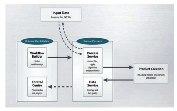
**Fig. 2:** Caris Onboard process flow diagram
