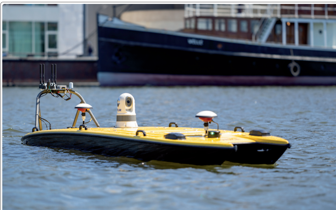
Fig. 3: The »Autonomous Surveyor« USV is ready to deliver high-speed hydrographic surveying as soon as new multibeam systems are available to provide this functionality
