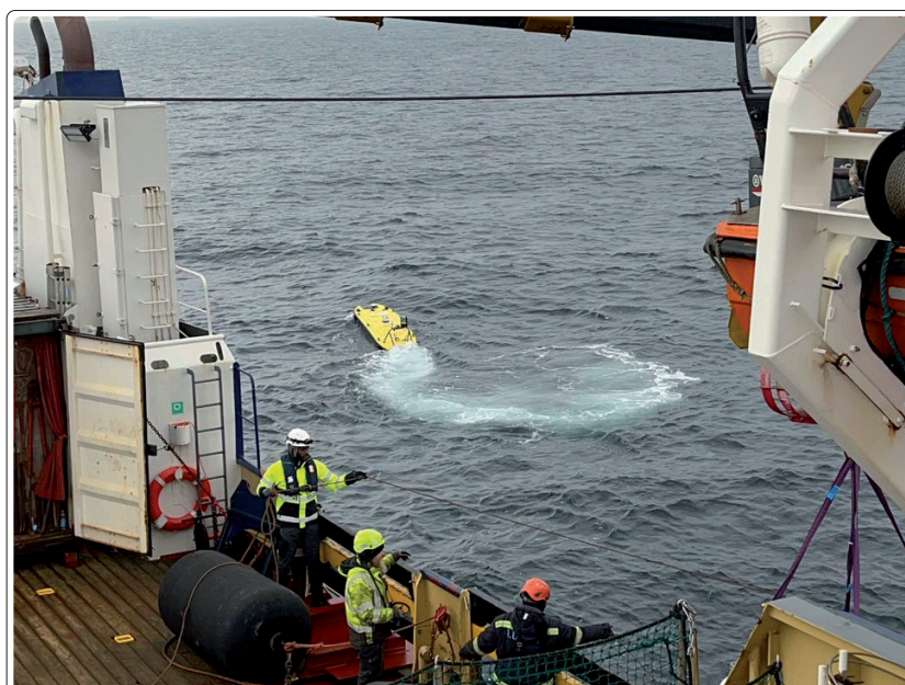
Fig. 4: A central mothership can be used to manage a single USV or a swarm consisting multiple survey platforms
