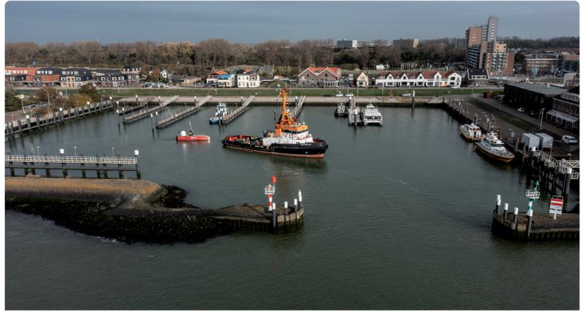
**Fig. 3:** Guard vessel accompanies the *Blue Essence* to comply with local regulations in the absence of dedicated legislation for uncrewed vessel operations
