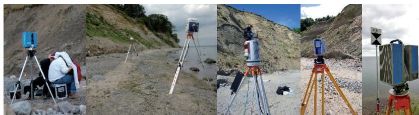
Fig. 2: Terrestrial laser scanning at the coastal cliff of Brodten – Z+F IMAGER 5003 (2004), Mensi GS100 (2005), Riegl VZ-400 (2010) and Faro Focus3D X330 and Z+F IMAGER 5010 (2016)
