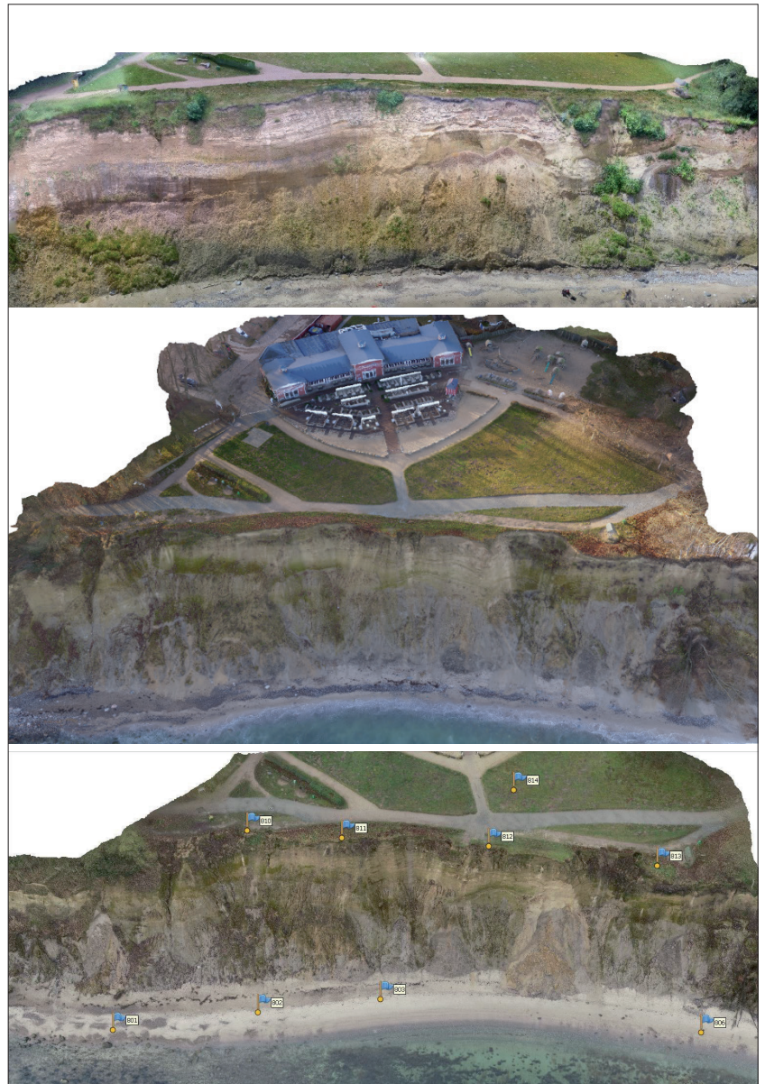
Fig. 4: 3D meshed models of the Brodten Cliff derived from UAS-based aerial imagery – June 2016 (top), December 2018 (centre) and January 2020 (bottom) including the configuration of nine ground control points (yellow dots with blue flags)
