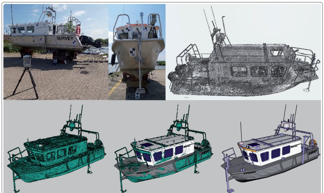
Fig. 2: Terrestrial laser scanning of the surveying vessel DVocean (top left and middle), the point cloud (top right) and the modelling process of the DVocean : from raw mesh (bottom left) to final model (bottom right)
