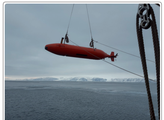
Fig. 3: The AUV of Université Laval (Quebec City) during its deployment in the Canadian Arctic off CCGS Amundsen
