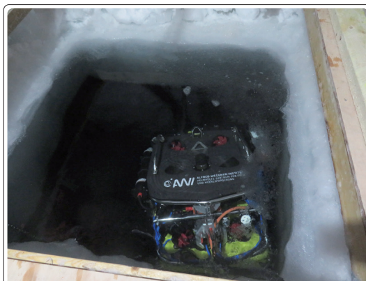
Fig. 2: The observation class ROV Beast deployed in its ice hole during the polar night of the MOSAiC expedition
