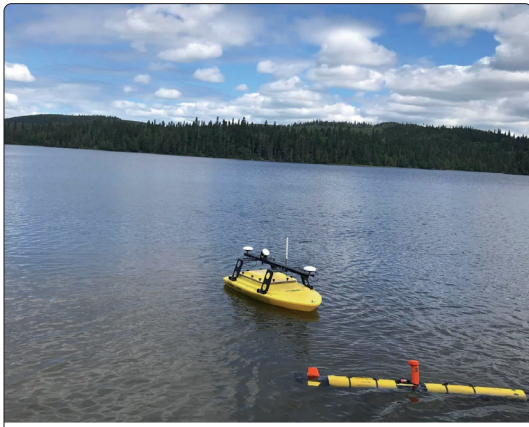
Fig. 7: Echoboat and AUV for automatics crab traps detection
