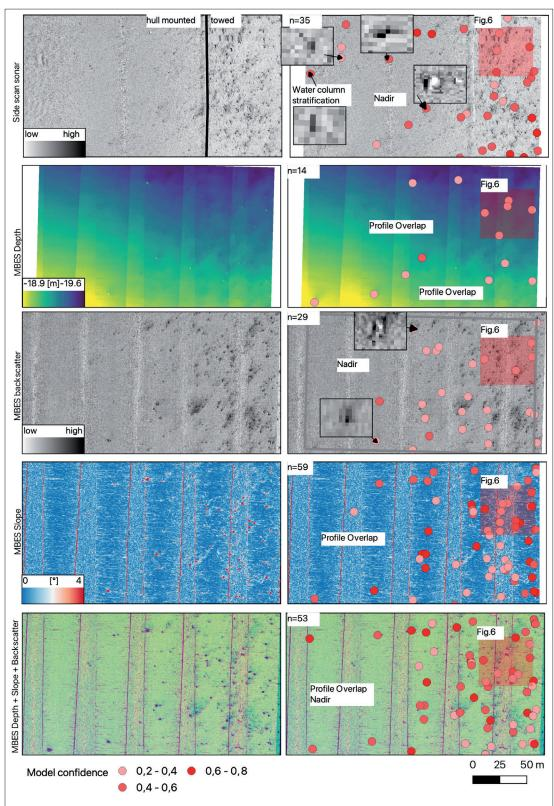
**Fig. 6:** Boulders found by the models in the test area in the different data sets. For the SSS backscatter mosaic, magnified insets show the similarity of small boulders and artefacts due to water column stratification and near-vertical incidence. Refer to Fig. 2 for location
