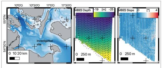
Fig. 1: Location of the investigation site west of Fehmarn (left). Water depths in the area range between 16 m and 25 m (centre), dashed lines are the survey lines run during MBES data collection. Right: Slope calculated from the local bathymetry
