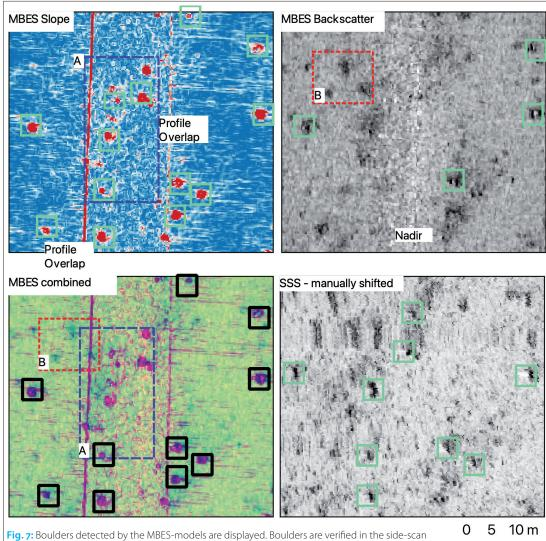
sonar image, whose position was shifted to account for positional inaccuracies. Near the nadir, potential boulders are not imaged in MBES backscatter data, while present in the slope map (blue rectangle). Vice versa, the backscatter map displays increased backscatter intensities in areas where no increased slope exists (red rectangle). No boulders are detected in both areas by the combined model working on depth-slope and backscatter channels. Refer to Fig. 6 for colour scales
