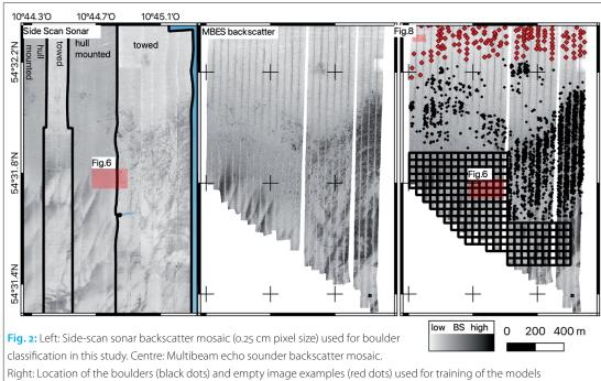
Right: Location of the boulders (black dots) and empty image examples (red dots) used for training of the models based on multibeam echo sounder data. The red box represents the test area for the manual identification of individual boulders in Fig. 6 and false positives examples in Fig. 8, respectively. The raster grid used for the manual determination of boulders densities is indicated
