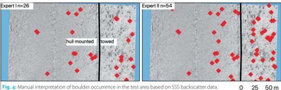
Fig. 4: Manual interpretation of boulder occurrence in the test area based on SSS backscatter data.
