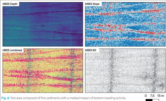
**Fig. 8:** Test area composed of fine sediments with a marked impact of bottom trawling activity. Because of the fine sediment composition, it can be assumed no boulders are present in this area. The model working on slope data detects several false positives in the area, while models running on backscatter, depth and the combined multi-band image report no false positives. Refer to the northwest of <u>Fig. 2</u> for location
