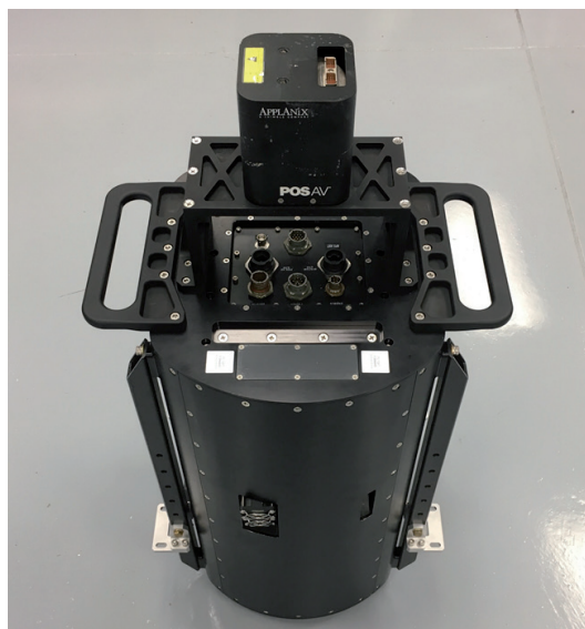
Fig. 2: RAMMS in »stack« configuration for use in manned aircraft missions
