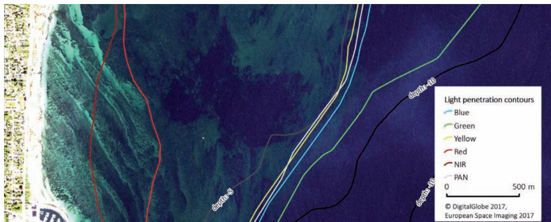
Fig. 1: Maximum light penetration depth of sunlight highlighted for the Baltic Sea (Denmark) using very high-resolution WorldView-2 satellite image data. The colours represent the different wavelengths of the sensor (colours) which are overlaid by 5 m and 10 m depth contours of the nautical chart. With increasing depth seafloor reflectance is dominated by shorter wavelengths. In organic rich waters such as the Baltic Sea the green wavelength(s) penetrate deepest
